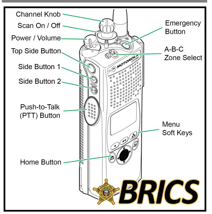
With the radio powered on, use the A-B-C zone select toggle switch and the 1 through 16 channel knob to select the proper talkgroup. The screen will display the zone letter and talkgroup name on the same line. Press and hold the PTT button to talk, and release to listen.
